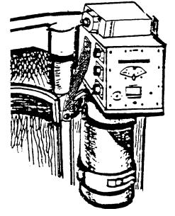
Control Console and Battery Box. Mounted in the 3-round vertical rack in the 152 mm conventional rounds storage area.
