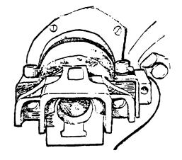
M240 Coax Machine Gun Microphone. On barrel jacket clamp.
