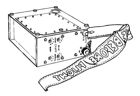
**3. Dispenser Assembly.** Attaches to the electronics module assembly or the external surface of the aircraft. It contains the breech, flare sensor, selector switch (C and F) for chaff or flare, reset switch, and housing. The housing contains the sequencer assembly which furnishes impulses to fire (in sequential order) each of the impulse cartridges.
