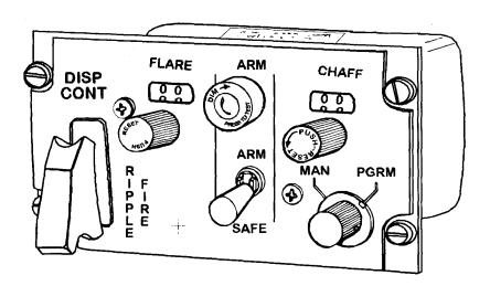
2. Electronics Module Assembly (EM). Attached either internally or to the external surface of the aircraft, it contains a programmer and a cable assembly which includes a 28-volt supply receptacle and a safety pin with flag assembly. On some aircraft installations the 28-volt supply receptacles and the safety switch have been relocated in the aircraft cable and are therefore remote from the EM.
